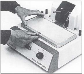
Two plates are supplied, each with two usable sides. When the plate is properly positioned, tighten the thumbscrew. (Figure 14)
